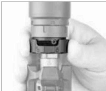
Verify the ASR collar is in the unlocked position before installing. Install the Velos LBP by sliding the back end over the muzzle device, then screw the silencer onto the muzzle device until it stops (hand tight, approximately 10-15 ft-lbs.). Rotate the ASR collar to the locked position. To remove, perform steps in reverse order.
