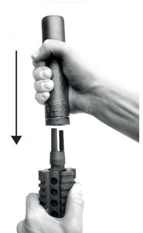
**Step 2-** Tighten the Saker firmly by hand until you cannot turn any further. Grip the textured suppressor body, not the MAAD Mount.
