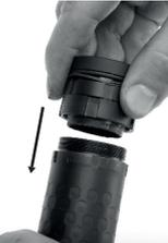
**Step 3-** Hold the suppressor body with a firm grip. Use the Multi-tool spanner cutout to tighten the coupler in a clockwise direction. To ensure the mount is completely tight, use the additional spanner tool to engage the slots in the suppressor body. Resume tightening the coupler with the Mutli-tool. The additional spanner tool will provide leverage. Torque to approximately 35 ft/lbs
