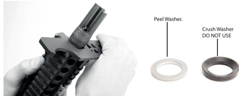
**NOTE:** Crush washers are NOT recommended as they do not crush uniformly and WILL cause improper mounting and baffle strikes. Silencerco recommends a peel washer if any clocking of the mount is required.
