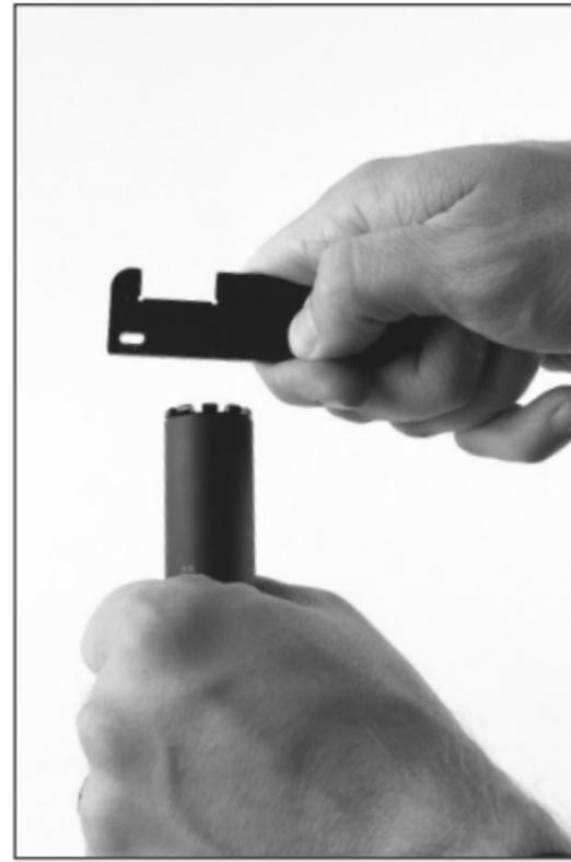
Inside the Warlock 22 or Spectre 22 back cap is an O-ring (Viton AS568-013), which seals the gases and debris from reaching the barrel threads of the host weapon and secures the suppressor during firing. This O-ring will need to be replaced from time to time. It is important to note that the Warlock 22 or Spectre 22 will function without the O-ring in place. The O-ring will need to be replaced once you notice a substantial amount of
