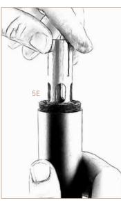
Slide baffle stack with attached expansion chamber into the silencer tube (4E), expansion chamber first, until it stops against the booster housing inside the tube.
