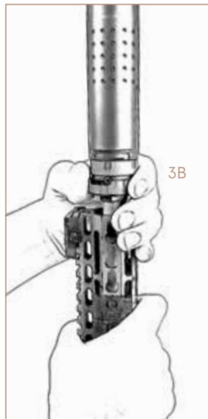
*CAUTION: Verify the ASR collar (3B) is in the unlocked position before installing. Installing the ASR Mount in the locked position may cause baffle strikes or other dangerous outcomes.*
